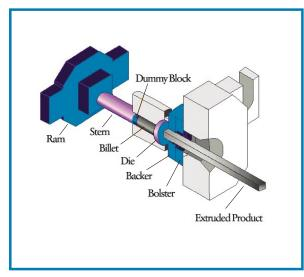
*Extrud-AL inerts all of the critical areas of the extrusion press in order to maximize life and reduce product surface defects.*
